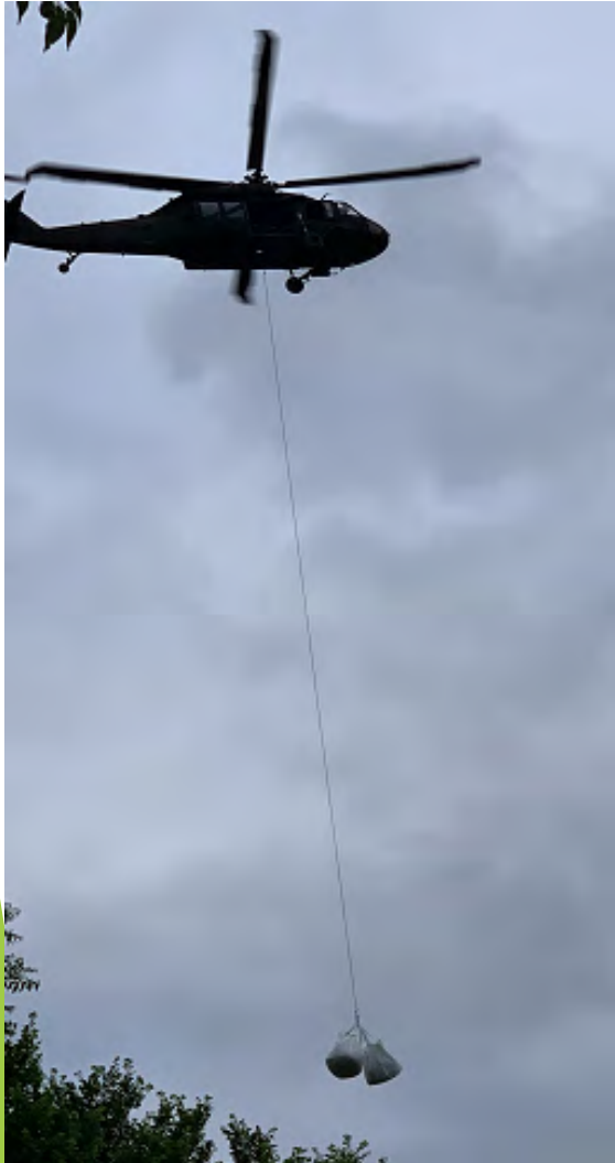
Dropping 3,000 lb. Sandbags
